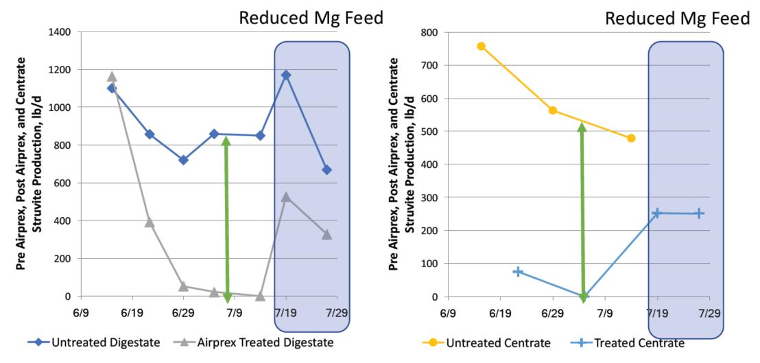
Significant reduction of struvite mass predicted between untreated and AirPrex® treated
