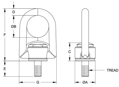
NOTE: ACTEC MODEL#56214 SP COIL, THREADS SHALL BE SECURED WITH LOCTITE RED 271
