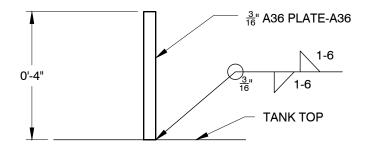
NOTE: SEAL WELD BOTH SIDES FOR BALANCE OF LENGTH AND GRIND SMOOTH
